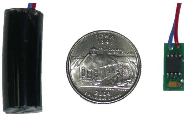
Figure 18. Photo of temperature sensor sealed in epoxy on the left. The temperature sensor on the right is identical to the one sealed inside of the epoxy. The twisted pair supplies ground along the blue wire and power/communication on the red wire.
