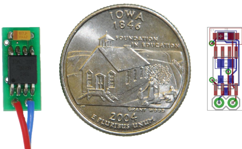
Figure 13. Photo of production temperature sensor with printed circuit board. There is one capacitor along the top, an ATtiny85V in the center, a two common-anode diode package and two resistors on the back. The twisted pair supplies ground along the blue wire and power/communication on the red wire.
